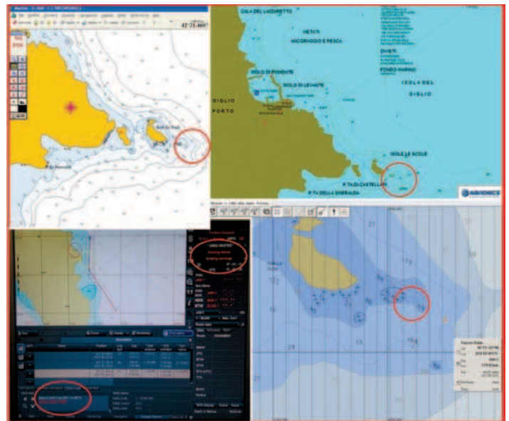
Figure 1 – Different electronic charts and the ECDIS system identify shallow water area and several alarms are activated
